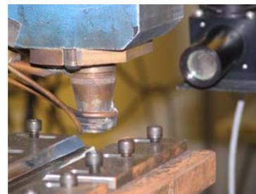
Figure 3 Laser welding setup
