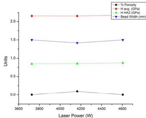
**Figure 5** Effect of laser power
