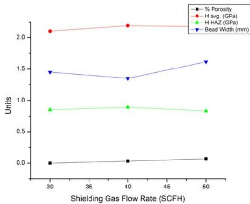
Figure 7 Effect of shielding gas flow rate
