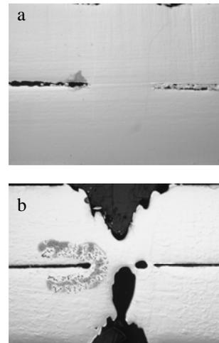
**Figure 4** Comparison of weld porosity a) weld made with copper alloying medium b) weld made without copper alloying medium
