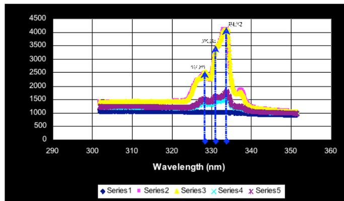
Figure 1: Comparison of zinc spectral intensity (Series 2 and 3: Without copper welds, Series 4 and 5: With copper welds)
