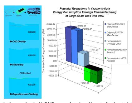
Energy reduction associated with DMD remanufacturing of large tooling in auto industry.
