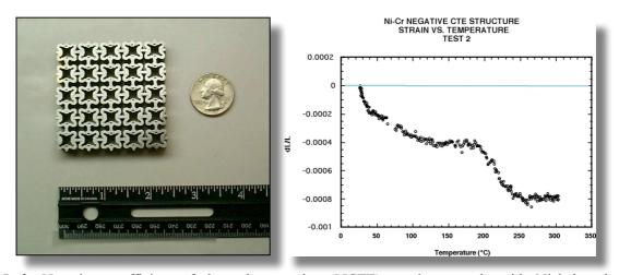
Left: Negative coefficient of thermal expansion (NCTE) specimen made with Nickel and Chromium by DMD process; Right: Behavior of negative strains of the NCTE structure in y-direction from a heating test in a precise controlled furnace.
