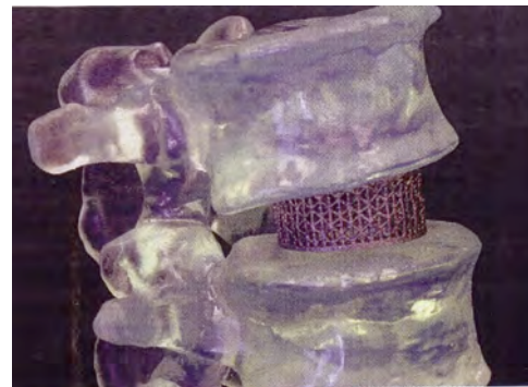
Model of spine showing a lattice cage implant produced using EBM technique ( www.orthosupplier.com )
